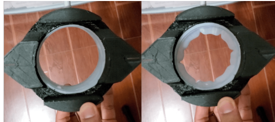
Fig. 5: Actual actuation with 30 kPa pressure yielding 28 mm of actuation.
